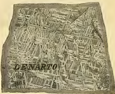
Fig. 3. SLAB OF CRYSTALLISED IRON FROM AEROLITE WHICH FELL AT LENARTO, HUNGARY.
